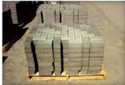
Figure 2. A cube of 90° herringbone pattern rectangular pavers ready for installation.
